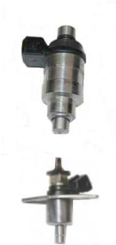
Mitsubishi Starion throttle body type Late 80's Turbo 2.6 Starion, Conquest, etc
